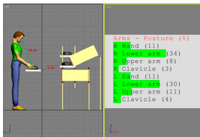
Figure 14. Body posture simulation of the 95th percentile male on workstation (a) designed to be optimal for the 5th percentile female. The distance of 68 cm from employee’s eyes to the work area was measured with the Tape tool.
